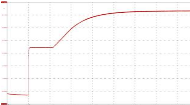
Figure 3: SPX78 start up response, V_{out}=5V
